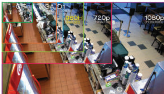
These images are examples of analog versus high-definition camera quality levels.
